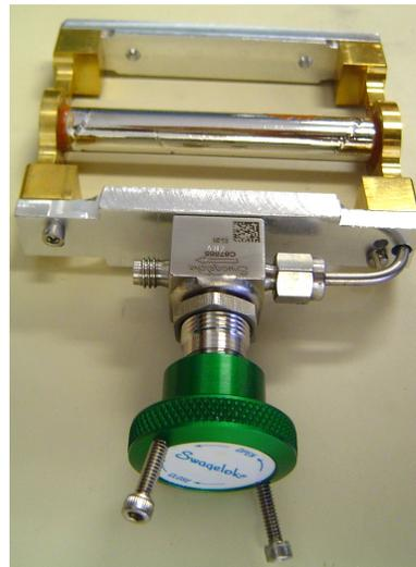
Figure 8.15: (Color online) A photograph of a prototype target cell filled with helium gas to 1.04 atm. The cell is 13 mm in diameter and 10 cm long.
