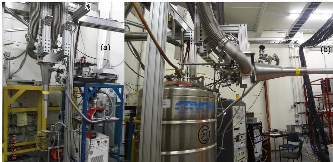
Figure 8.1: (Color online) A target stand supports the dilution refrigerator on the beam line both (a) vertically for target changes and (b) horizontally for operation.
