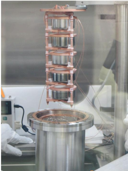
**Figure 2.3:** (Color online) A string of broad-energy germanium detectors for the prototype module that were assembled underground.
