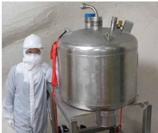
**Figure 2.2:** (Color online) Custom liquid-nitrogen Dewar that is part of the cryogenics system that will cool the detector arrays.
