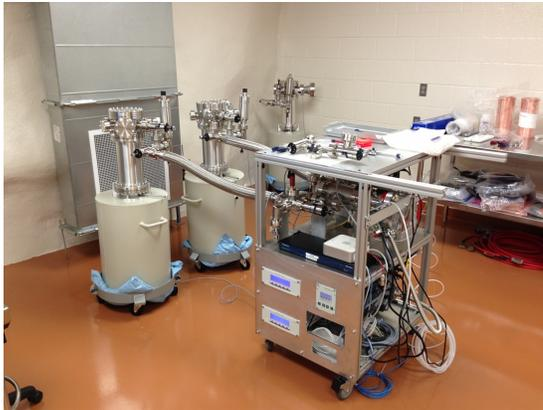
Figure 2.9: (Color online). The STC pump-cart connected to two STCs.
