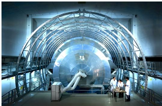
Figure 2.32: (Color online) The KATRIN main spectrometer and the air coil system.
