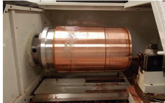
**Figure 2.4:** (Color online) Cryostat 1 being machined from electroformed copper at the underground machine shop.
