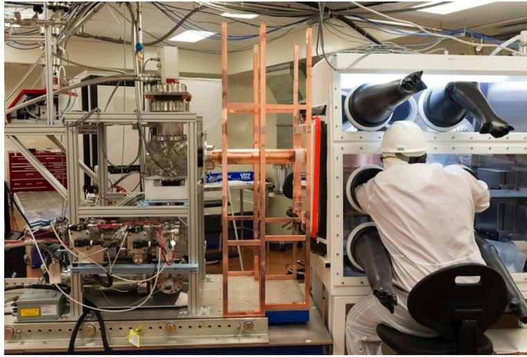
Figure 5: (Color online) Majorana collaborators work inside of a special low-radon, class-10 glove box to install a string of natural HPGe detectors in the prototype cryostat. The associated vacuum system is to the left in this photograph.
