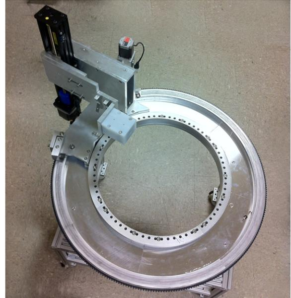
**Figure 8.41:** A picture of the actual calibration stand as it was nearing completion. The detector Dewar will be centered in the circular track.
