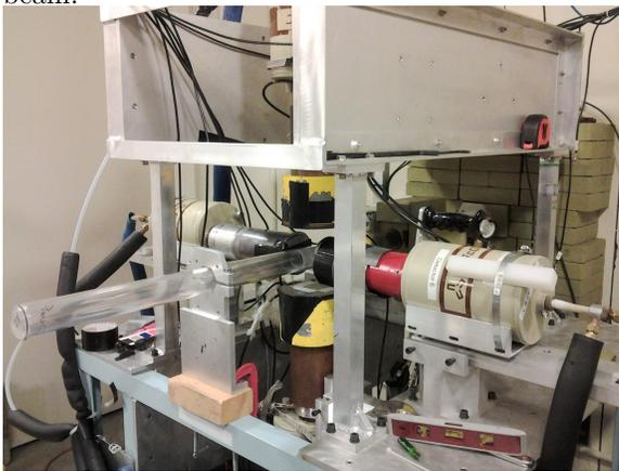
Figure 6.1: (Color online) Experimental setup with two detectors at  $90^\circ$  in the plane of beam polarization and two detectors in the plane perpendicular to the plane of beam polarization.
