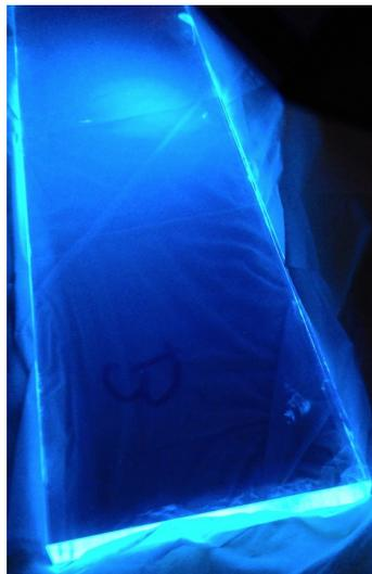
**Figure 1.11:** (Color online) An acrylic plate swing-coated with protonated PS and TPB for the ORNL light-collection measurements. A UV lamp is used to cause the observed fluorescence.
