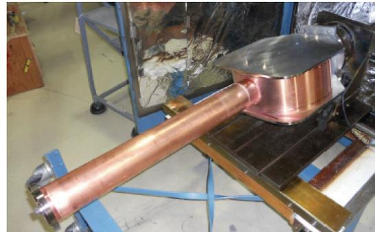
**Figure 2.5:** (Color online) Cryostat 1 parts during welding at PNNL.
