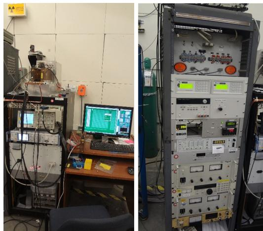
Figure 8.10: (Color online) Preparation for the second cool-down. The left photograph shows the NMR system; the right one shows the electronics rack for the thermal sensors, the LHe level readouts, etc.
