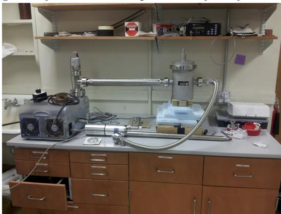
**Figure 2.18:** (Color online) Setup for pumping of the Melissa detector.
