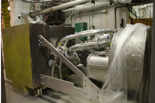
**Figure 8.37:** (Color online) Partially assembled heavy-water tank and cryostat on the thermal column door, rolled out of the reactor thermal column void.
