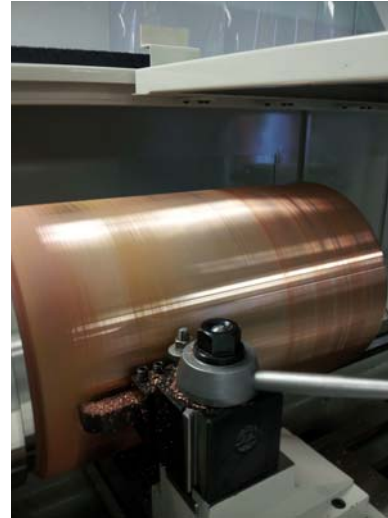
Figure 2.5: (Color online) Machining of electroformed copper on the lathe
