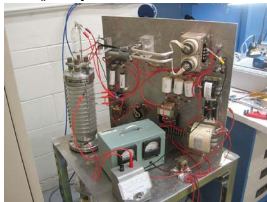
Figure 7.25: (Color online) Ion-source test stand with its cover removed to show the accelerator tube, electronics, and metering gauges.
