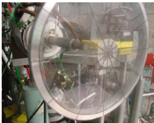
Figure 4.6: (Color online) ^{181}\text{Ta} target placed in front of the deuterium gas cell.
