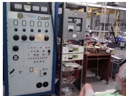
Figure 8.4: (Color online) Photo of microwave system test; EIO powered by Cober.
