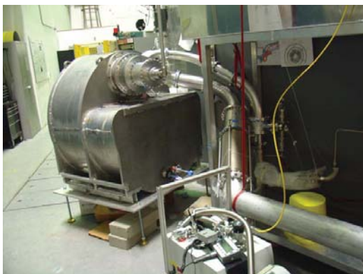
Figure 8.15: (Color online) Photograph of the large aluminum container that houses the \text{D}_2\text{O} thermal moderator surrounding the UCN source assembly. The UCN source is located within this container.
