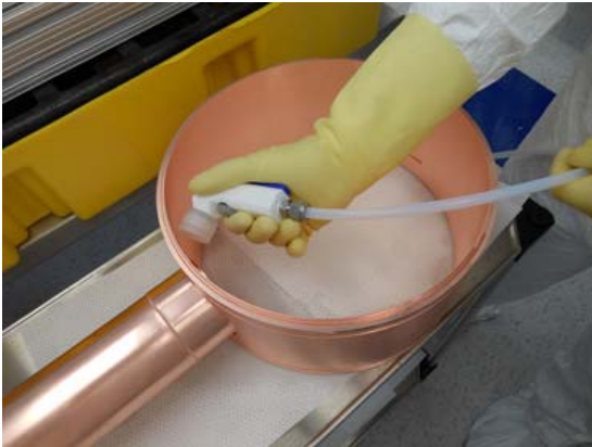
Figure 2.9: (Color online) A copper part being dried with purified liquid nitrogen boil-off after it had been etched and passivated.
