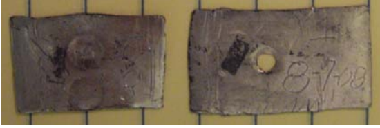
Figure 2.15: (Color online) The two aluminized non-low-background lead shims that were removed from MALBEK. They were located between the high-voltage copper foil and the germanium crystal. Together the shims contain 3.013 g of lead.
