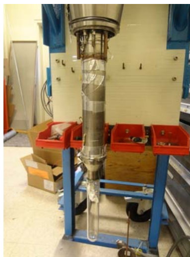
Figure 8.1: (Color online) A newly developed, \text{LN}_2 -tested mixing chamber mounted to a dilution refrigerator.
