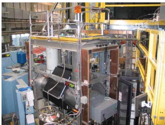
Figure 1.9: (Color online) The neutron lifetime apparatus on the NCNR beamline.
