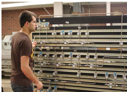
Figure 8.17: (Color online) Photograph of the methane and deuterium gas-handling systems.
