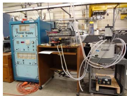
Figure 8.5: (Color online) Photo of microwave system test; carcinotron powered by Siemel.
