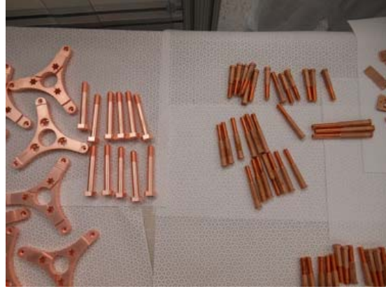
Figure 2.10: (Color online) To the left are copper parts after they have been etched, passivated and dried. To the right are copper parts before any cleaning.
