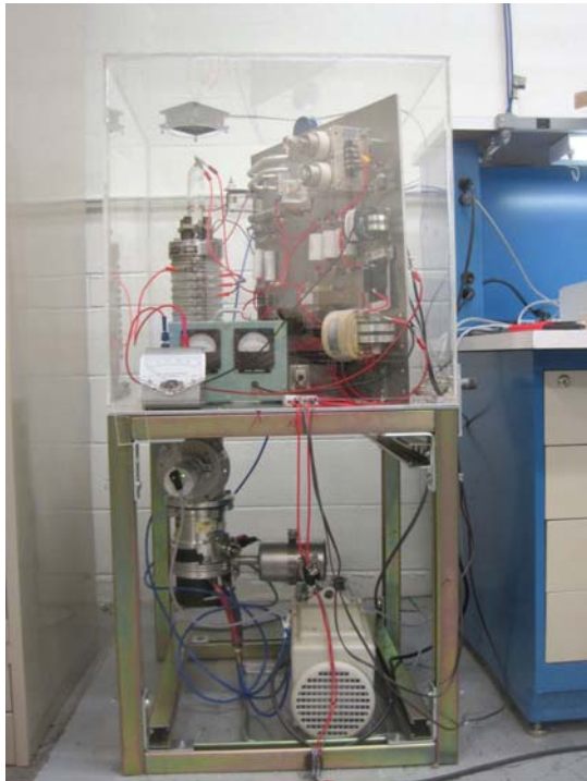
Figure 7.24: (Color online) The new ion-source test stand with its protective cover in place.
