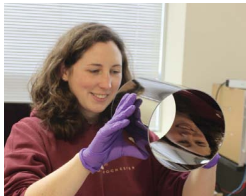
Figure 8.16: (Color online) Photograph of a ^{58}\text{Ni} -coated neutron guide that resides in the UCN source assembly.
