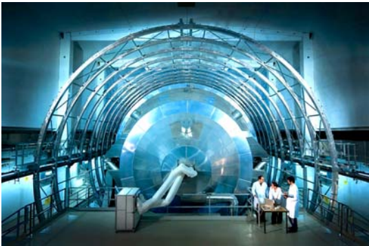
Figure 2.36: (Color online) The KATRIN main spectrometer and the air coil system.
