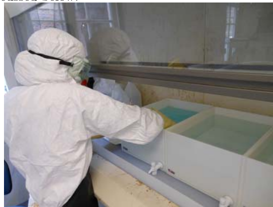
Figure 2.8: (Color online) Etching a copper part in the cleanroom hood. A copper part is being scrubbed in the sulfuric acid bath. The bath is initially clear; the blue color is from copper sulfate. To the immediate right of the sulfuric acid bath is the first rinse bath, followed by the citric acid bath. Not pictured is the second rinse bath.
