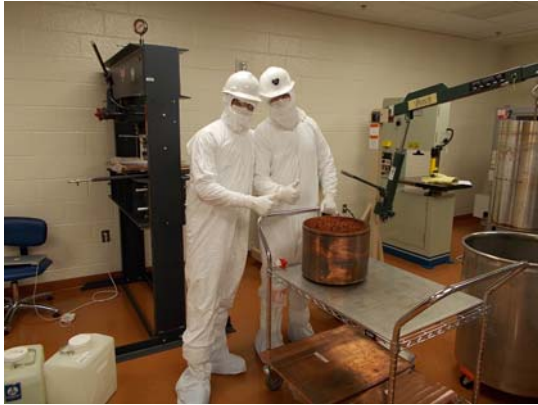
Figure 2.4: (Color online) A completed bottom lid for one of the DEMONSTRATOR cryostats
